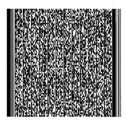
Figure 3: PDF417 encoding of Abraham Lincoln's Gettysburg Address
